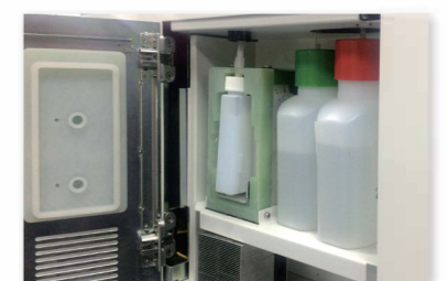
Built-in CRP reagent cooling system
